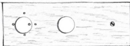
2. After each exposure, advance the film by turning the Film Advance Knob (D) one-and-a-quarter revolutions for the first five shots. After those first five shots, the dot of the Film Advance Knob (D) will align with the uppermost marking on the top cover.
